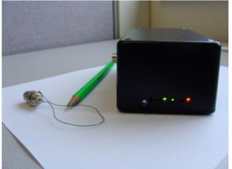
Our credit card cloner is constructed from a single board linux computer, a small custom circuit constructed from cheap (less than \$10) ubiquitous components, and a device driver of our own authorship. A diagram and parts list will be made available at the same time as the submission of the full version of our paper. A version of our device driver will also be made available, although certain details will be redacted in order to prevent illegal use by the unethical.
